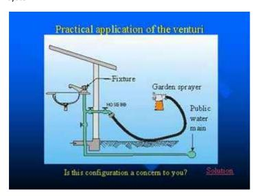
Back siphonage is a practical example of the venturi effect, essentially the same as sucking liquid through a straw.
