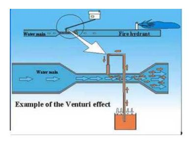
Backsiphonage can occur when there is reduced pressure in the distribution pipes created by an interruption in the water supply, such as a main break or repair, or increased water velocity within the pipes created when there is a large draw such as fire fighting, or flushing through hydrants., and creating higher than normal water velocity in the distribution pipes.
