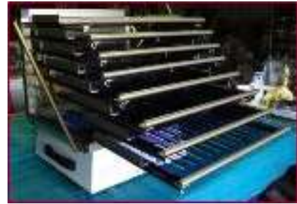
Medium Orbital/Cyclic Platelet Shaker set up with 8 shelves shown in the loading position.
