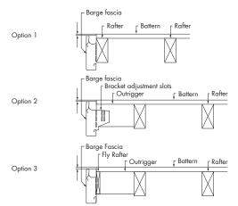
Cut both ends of the barge at an angle to suit the pitch of the roof. A Barge mitre is used to finish the joint between the barge and the Fascia. At the roof apex the 2 Barge lengths are joined by leaving a flange on one which inserts into the other and is secured by blind rivets.
