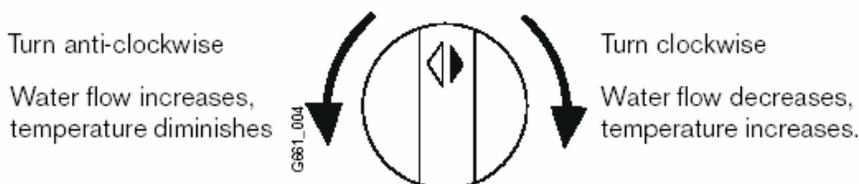
Turn anti-clockwise Water flow increases, temperature diminishes
