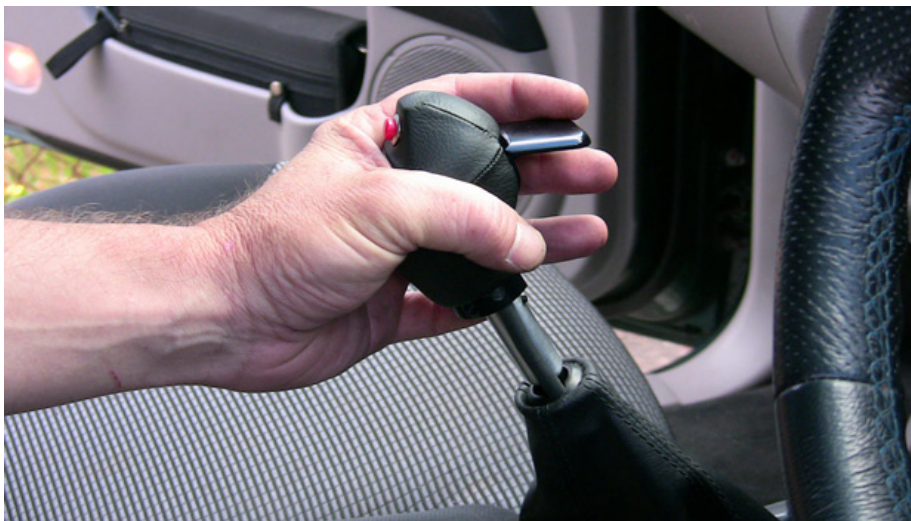
The duck clutch hand operated clutch system
