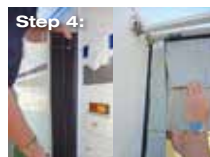
Step 4: Install wall rail uprights to seal the ends against the van
