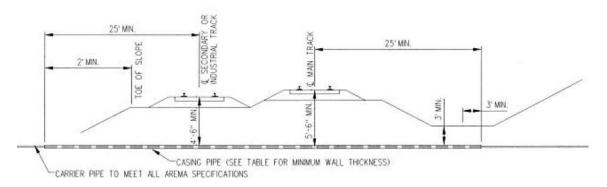
ALL MINIMUM DIMENSIONS MEASURED NORMAL TO & OF OUTSIDE TRACK.
