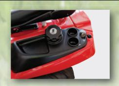
Convenient side panel including an auxiliary power outlet (12v), drink holders and a large fuel cap with a fuel level indicator.
