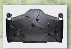
The performance comes from this heavy duty 8 gauge mulching deck. 6 blades with 12 cutting tips makes for fast, efficient cutting and mulching. The cut and mulched grass is discharged from the rear of the cutting deck, clean and tidy.
