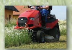
This mulching deck can manage high grass with ease. The chains trap and hold the cut material within the cutting area, allowing the 12 blade tips to reduce the longer grass down to a mulch.
