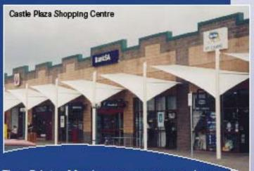
The Fabric Membranes can span large distances without supporting structure used in conventional building. Galvanised and powdercoated steelwork, stainless steel corner plates and wire cables, combined with the membrane, create virtually maintenance free covered areas which protect against harmful U.V. rays and the elements.
