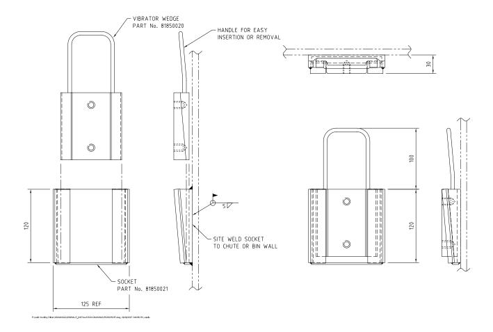
Wedge mount is specifically designed for use where permanent mounting of the vibrator is not possible.
