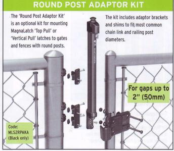
Post diameters: 17/8"-2" (48-50mm), 23/8" (60mm), 27/8" (73mm) Gate diameters: 13/8" (35mm), 15/8" (41mm)
