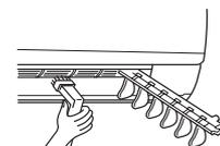
4. Put the vertical vanes back to their original positions correctly one by one, into their respective guide.
