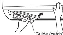
5. Install the horizontal vanes by following the removal procedure in reverse.
