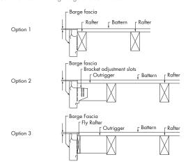
Cut both ends of the barge at an angle to suit the pitch of the roof. A barge mitre is used to finish the joint between the barge and the fascia. At the roof apex, the 2 barge lengths are joined by leaving a flange on one which inserts into the other and is secured by blind rivets.
