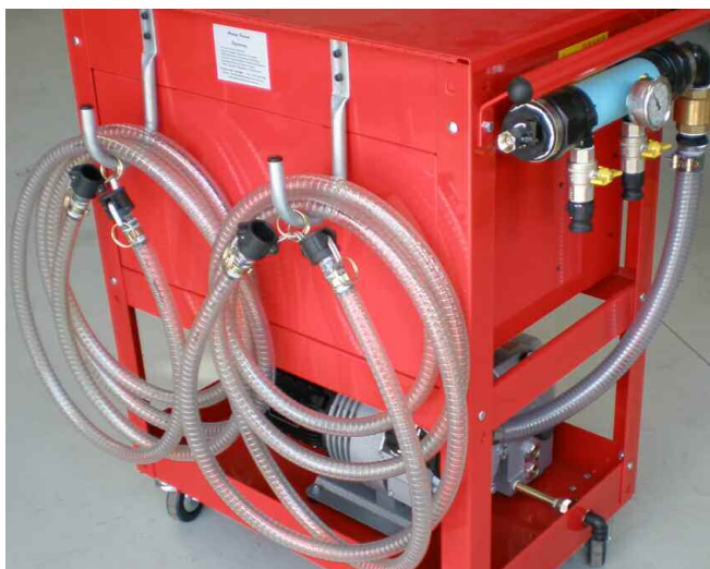
AVE Manifold and Catchpot Hoses with Camlock Fittings- Makes connecting pumps and Manifolds and Catch-pots a snap!
