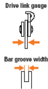
Figure 35: Drive link and bar groove must match.
