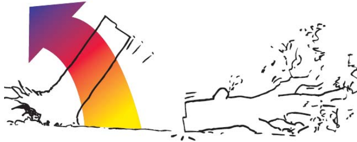
Figure 83: Beware of stump springing back
