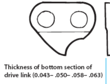
Figure 36: Drive link gauge
