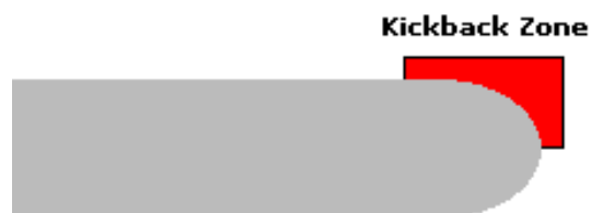
Figure 60: Kickback reaction zone
