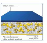
The inner blanket forming the core of Trithor is a truly unique blend of fibres that add to the durability and effectiveness of Trithor Termite Protection.
