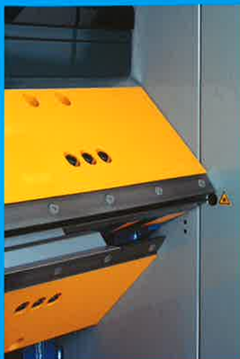
Detail of bending apron
