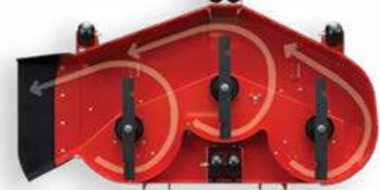
TUNNEL GEOMETRY - An advanced cutting chamber is formed by setting the blades back four inches from the front of the deck for less clumping and even grass dispersion.
