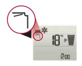
Scene 2: Declines to a maximum 0° angle. Sets vane angle to lowest position: Optimised for gentle airflow heating.
