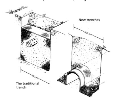
The failure of the trench is a common cause of problems with onsite sewage management systems. Trenches usually fail if the holes in the pipes that run through the trenches get blocked up, or if the effluent is unable to evaporate or drain away. You can tell if the trench has failed because the area will be soggy, smelly and covered with profuse grass growth.
