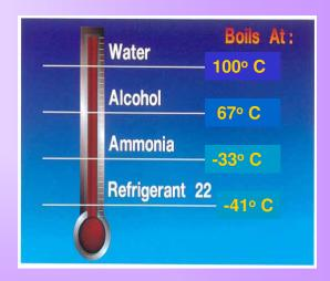
Because R-22 is one of the refrigerants commonly used in air conditioning, we'll use it in an example to see just what happens inside the cooling coil.
