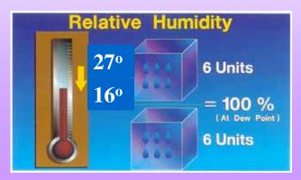
At the dew point, the air is holding all the moisture it can for that temperature; or to put it another way, the relative humidity is 100%.
