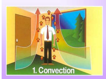
When heat is given off by convection, the air close to the body becomes warmer than the air away from the body. Since warm air is lighter than cool air, it floats upward. As it does, it is replaced by the cooler air. As this cooler air absorbs body heat, it too floats upward.
