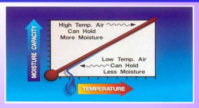
Because relative humidity has a direct correlation to temperature, any time the temperature is raised or lowered, the relative humidity or moisture content of the air will also change. Cool air has less capacity to hold moisture than does warm air.
