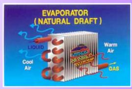
through the coil, until it's completely vaporized.
