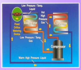
liquid, and the metering device reducing the pressure to convert the hot liquid into a cold liquid entering the evaporator.
