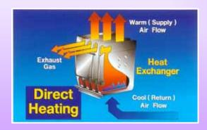
A popular method is "direct" heating, where heat supplied by burning either gas or oil is transferred to the room air through a metal heat exchanger in a furnace.
