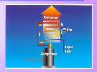
The heat removal process causes the refrigerant to return to a liquid state as it leaves the condenser, moving toward the metering device in the liquid line.
