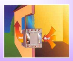
It's easy to think of an air conditioning system as something that produces "coldness." Actually, it is more accurate to think of it in terms of removing heat. The heat in a room is transferred to the cold refrigerant flowing through an air conditioner coil.
