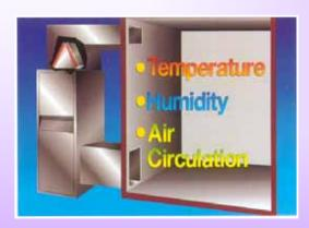
Changing the conditions that affect comfort is the job of the air conditioning system, a system for controlling air motion and either adding or taking away heat and humidity.
