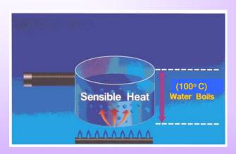
To understand the principle, we'll start with a pot of water. As the water absorbs heat, its temperature rises until it reaches the boiling point of 100° C.
