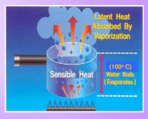
This physical principle is one key to operation of refrigeration systems ... the ability of a liquid to absorb a large amount of heat as it vaporizes.
