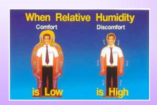
When the surrounding air has a low relative humidity, the body is able to give off more heat through evaporation.
