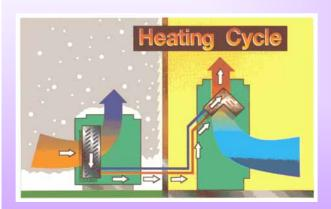
During the heating season, heat is moved from the outdoor air, through the same refrigerant system, to the indoor air.
