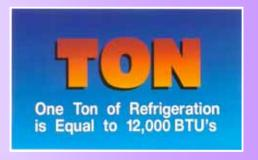
A TON of cooling capacity is equivalent to the amount of heat required to melt one ton of ice at  $0^{\circ}$  C (32' F) in a 24-hour period. One ton of refrigeration is equal to 12,000 BTU's per hour. A ten-ton rooftop unit has a cooling capacity of 120,000 BTU's per hour (35 kW).
