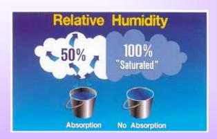
For example, when we say that the air has a relative humidity of 50%, we are saying that the air at this specific temperature contains half the amount of moisture it can actually absorb.
