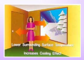
The temperature of surrounding surfaces is also important because it affects the rate of radiation. The lower the temperature of the adjacent surface, the more cooling effect the body will feel through radiation.
