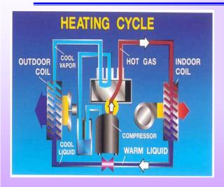
When heating is required, the reversing valve routes the hot gas discharge from the compressor to the indoor coil which now acts as a condenser. The heat given off by the refrigerant as it condenses is transferred to the relatively cooler indoor space.
