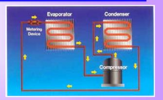
We need a compressor, a metering device, and some type of condenser. These parts move the refrigerant and regulate its flow in a process that removes the heat that has been absorbed by the refrigerant, enabling the evaporator to use the refrigerant over and over.
