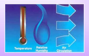
Temperature, relative humidity, and air motion are three conditions that affect the body's ability to reject heat.
