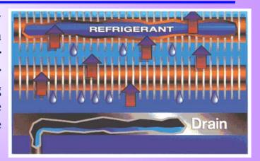
At the same time, water vapor condenses on the coil. That is, it turns into liquid water, which is then drained off. In order to understand what causes this condensing, or dehumidifying, action, we need to look a little closer at "relative humidity."
