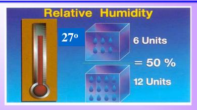
Relative humidity, as you will recall, is a measure of the actual moisture content of air in relation to its capacity to hold moisture. So, if the air in a 27° C room is capable of holding 12 units of moisture per cubic foot, and its actual moisture content is six units, its relative humidity is 50%.
