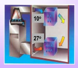
The same thing happens with a cooling coil. When the air around it is saturated with moisture, the excess moisture condenses on the coil. From there, it is drained out of the system. The air supplied to the house at 10° C is cooler and drier than the 27° C return air.
