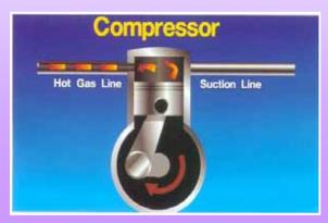
This is a critical step in the process, because the refrigerant must be hotter than the outside air in order for heat transfer to occur at the condenser.
