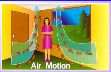
Air motion also speeds up the convection process by removing the warm air close to the body and carrying away the heat that's been given up. Air in motion may also remove heat from walls, ceilings, and other surfaces surrounding the body.
