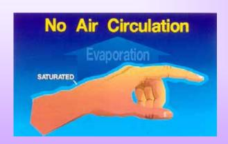
If there were no air motion, the layer of air closest to the body would soon approach saturation. Its relative humidity would increase to the point where it could no longer absorb water vapor.
