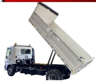
**ALDOM Tippers** are designed for today, focussed on tomorrow, Aldom tippers are designed and built from high-quality materials to make them tough. Our tippers can be made from Hardox or normal mild steel and are fitted with rails, access steps, headboard guards, and two-way hinged air operated tailgates.
