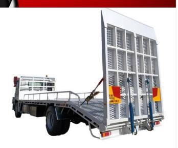
**ALDOM Trays** are built tough, designed for the harshest of Australia's environments, fitted with tie rails, cab height headboard with 600mm high bash plate, 30mm coaming lip, access steps both sides front and rear with an underrun bar to suit the rear (tow bar independent). Aldom Transport Engineering can also supply split or one-piece dropsides.
