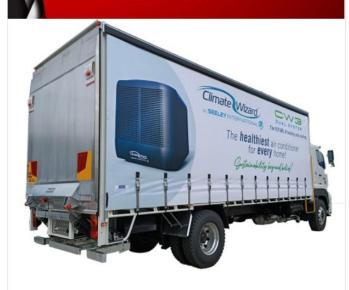
ALDOM Tautliners / Curtain Siders have heavy-duty front walls, single sheet aluminium roof with ply underneath and can be insulated. They are stitch welded around the floor to the coaming rail with 30mm lip (unless not required). Each unit is provided with access steps and fitted with 'Barn Doors', four hinges and cam locks.
