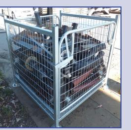
Small items are kept Ensure load can be safely unloaded by the receiver secure in the correct size mesh stillage
