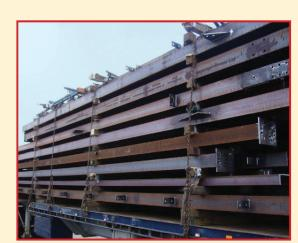
Insufficient load restraints for load being carried
