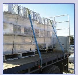
Items should be suitably and securely strapped (and/or wrapped) when being transported on pallets
