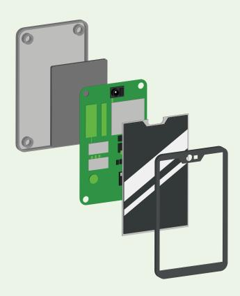
Mobile phones are disassembled into component parts, which are then transported to local and overseas recyclers for processing. The plastic can be made into shipping pallets and lithium extracted from the phones can be made into new batteries.
