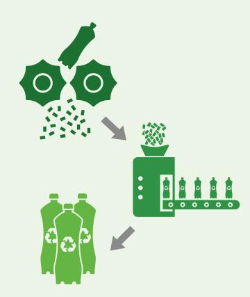
Next, all of the bottles are ground up and shredded into flakes. Finally, they are melted down and formed into small pellets, each about the size of a grain of rice. The pellets are bundled up and sold to companies that can melt them and make them into many different products.
