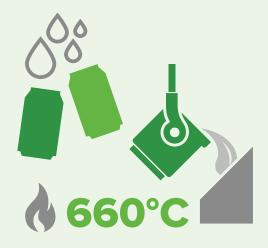
All cans are washed then melted down to molten aluminium at a temperature of 660°C to remove any ink from the cans.
