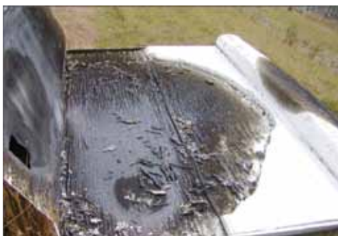
(PHOTO 1) EPS PANEL AFTER DIRECT EXPOSURE TO 300KW FIRE FOR 60 MINUTES AT BRANZ.
