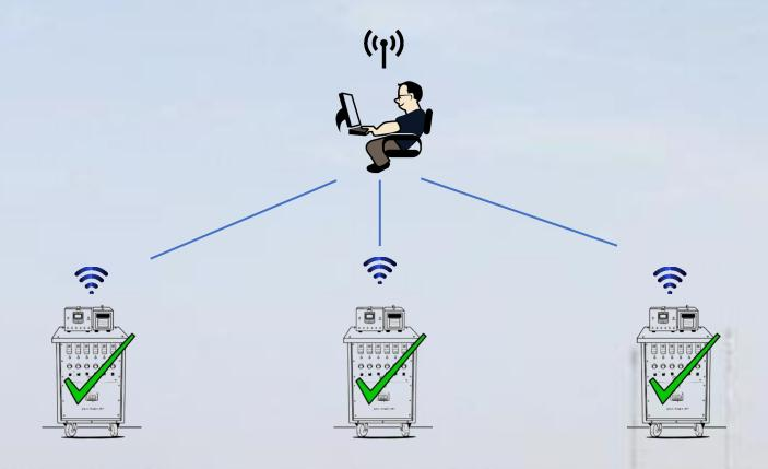
Multiple work fronts can be simultaneously monitored from an on-site remote safe-haven, using a computer connected via Heat Tech's RMS Network. The network consists of long-range Wi-Fi transceivers, which can be installed with repeater stations to suit any on-site application.
