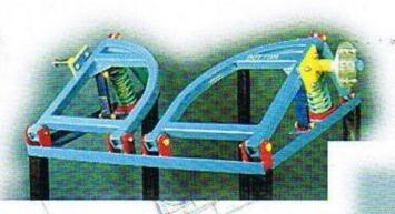
Martin's Trailer Parts have been manufacturing quality parts for the trailer industry for over 25 years and are now proud to introduce their Gaffa Suspension for use on and off road. The suspension features a progressive load coil spring designed to give greater support to
