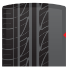
Irregular shoulder wear (unbalanced/misaligned)
