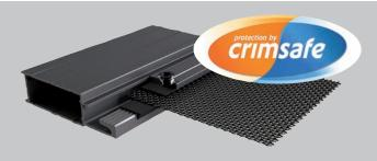
All Crimsafe® doors feature a unique Screw-Clamp™ system. Tamper resistant screws go through a metal clamp then through the Tensile Tuff security mesh and is then driven right into the frame to hold the mesh in a vice like grip which gives the door enormous strength against attack. Crimsafe® doors are the only security system to feature the unique Screw-Clamp™ design for unbeaten strength.
